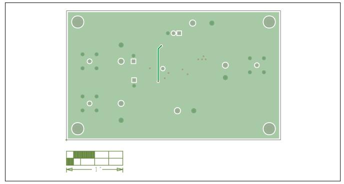
Figure 4. MAX44291 EV Kit PCB Layout—Component Side
