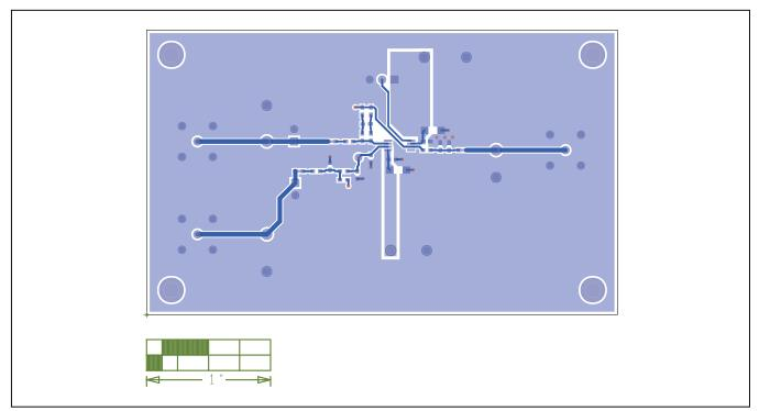
Figure 3. MAX44291 EV Kit PCB Layout—Component Side
