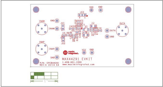
Figure 2. MAX44291 EV Kit Component Placement Guide—Component Side
