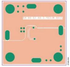
Figure 12. Bottom Layer, Recommended Layout for WLCSP
