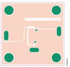
Figure 13. Bottom Layer, Recommended Layout for TSOT
