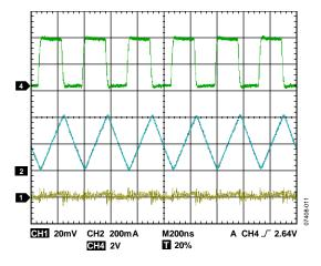
Figure 8. PWM Operation at Medium Load (1.8 V Model)
