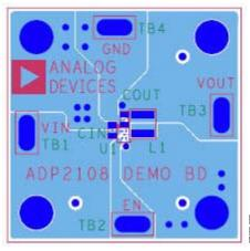
Figure 10. Top Layer, Recommended Layout for TSOT
