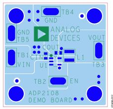
Figure 11. Top Layer, Recommended Layout for TSOT
