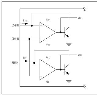
Figure 2. Simplified Model of a Logarithmic Amplifier
