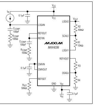
Figure 6. Dual-Supply Typical Operating Circuit
