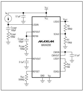
Figure 5. Single-Supply Typical Operating Circuit
