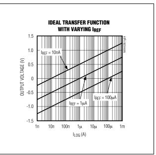
Figure 4. Ideal Transfer Function with Varying IREF
