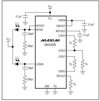
Figure 7. Measuring Optical Absorbance
