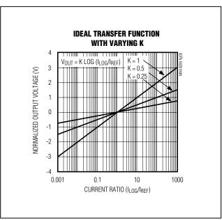
Figure 3. Ideal Transfer Function with Varying K
