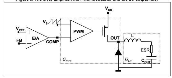
The transfer function on the LC filter is given by:
