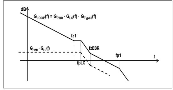
Figure 14. Open loop gain: module Bode diagram
