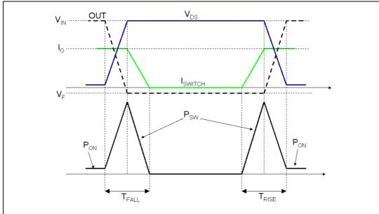
Figure 16. Switching losses
