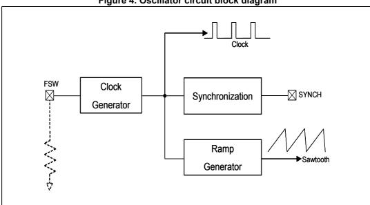
Figure 4. Oscillator circuit block diagram
