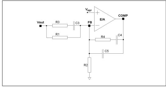
Figure 10. Type III compensation network
