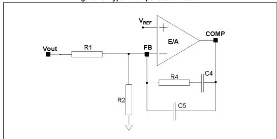
Figure 13. Type II compensation network
