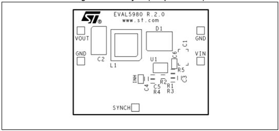
Figure 20. PCB layout (bottom side)
