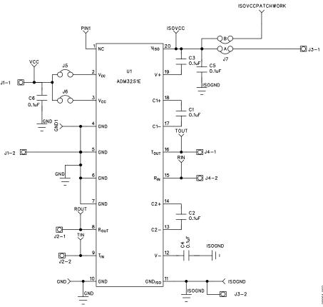
Figure 2. Schematic of the ADM3251E Evaluation Board
