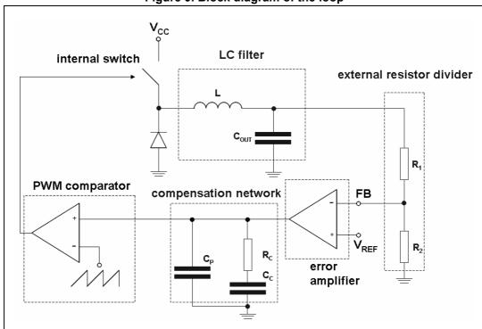
Figure 9. Block diagram of the loop
