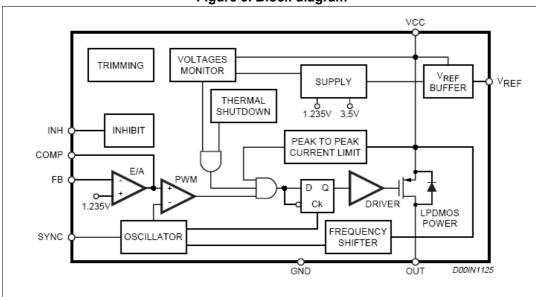
Figure 3. Block diagram
