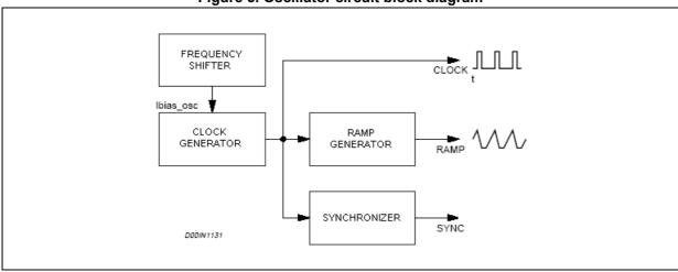
Figure 5. Oscillator circuit block diagram
