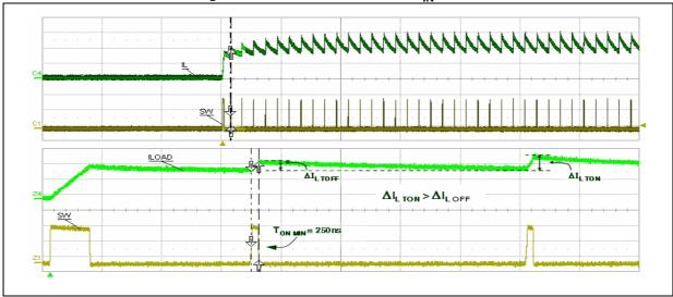
Figure 17. Short-circuit current  $V_{IN}$  = 36 V
