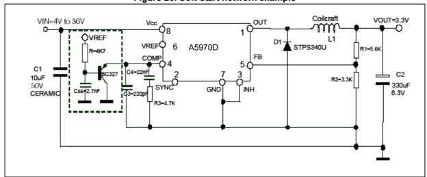
Figure 26. Soft-start network example
