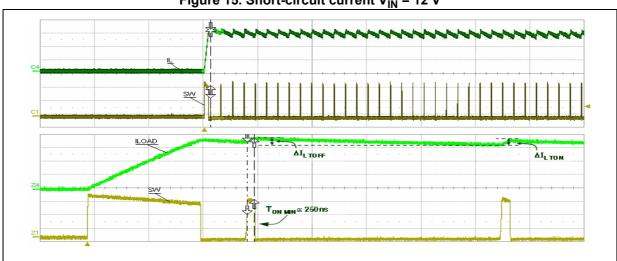
Figure 15. Short-circuit current  $V_{IN}$  = 12 V
