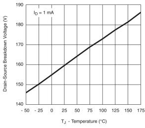
**Drain-Source Breakdown vs. Junction Temperature**
