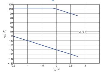
Figure 26: Measuring range versus external  $V_{\mathrm{ref}} \mathrm{LXSR}$  25-NP
