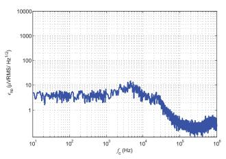
Figure 9: output noise voltage spectral density
