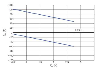
Figure 25: Measuring range versus external  $V_{\mathrm{ref}}$
