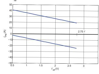
Figure 24: Measuring range versus external  $V_{\mathrm{ref}}$
