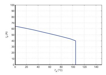
Figure 16:  $I_P$  vs  $T_A$  for LXSR 6-NPS
