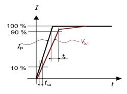
Figure 22: Response time  $t_r$  and reaction time  $t_{ra}$
