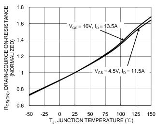
Figure 6. On-Resistance Variation with Junction Temperature
