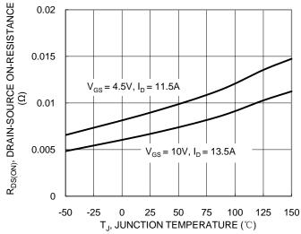
Figure 7. On-Resistance Variation with Junction Temperature
