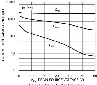
Figure 10. Typical Junction Capacitance
