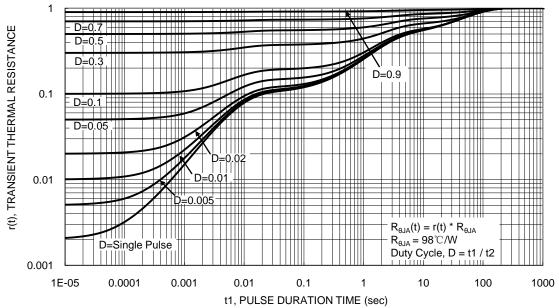
Figure 13. Transient Thermal Resistance
