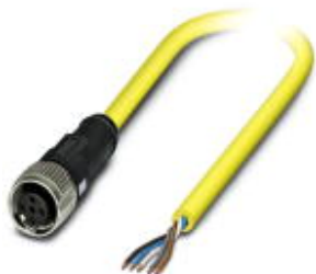
Sensor/actuator cable, 5-position, PVC, yellow, free cable end, on Socket straight M12 SPEEDCON, A-coded, cable length: 5 m
